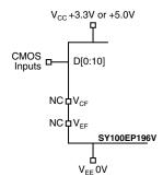
Figure 9c. Connecting CMOS Signals to the D Inputs
