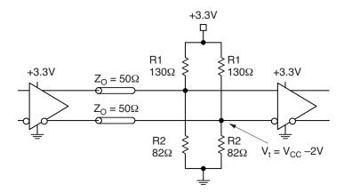
Figure 6a. Parallel Termination—Thevenin Equivalent
