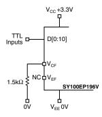
Figure 9d. Connecting TTL Signals to the D Inputs with  $V_{CC} = 3.3V$
