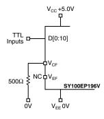
Figure 9e. Connecting TTL Signals to the D Inputs with  $V_{CC} = 5.0V$
