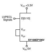
Figure 9b. Connecting LVPECL Signals to the D Inputs
