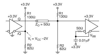
Figure 6c. Terminating Unused I/O
