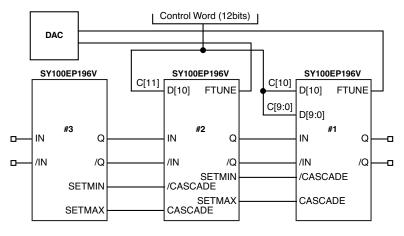
Figure 10b. Cascading Three SY100EP196V
