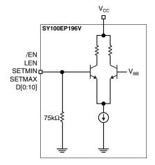
Figure 1b. Single-Ended Input Structure
