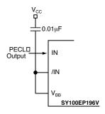
Figure 7a. Interfacing to a Single-Ended PECL Signal
