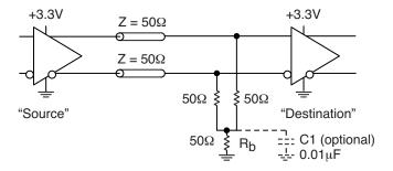
Figure 6b. Three-Resistor "Y-Termination"
