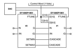
Figure 10a. Cascading Two SY100EP196V
