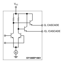
Figure 2. Emitter Output Structure
