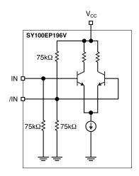
Figure 1a. Differential Input Structure
