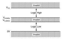
Figure 4b. Input Levels, CMOS, TTL
