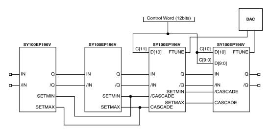
Figure 10c. Cascading Four SY100EP196V
